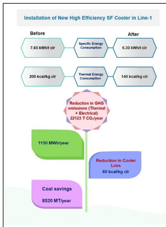
Figure 7.2: Impact of Installation of new high efficiency SF cooler in Line-1
